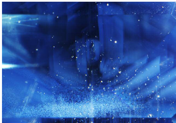
Figure 62. Zircon crystals scattered throughout angular milky clouds were more prominent in these sapphires compared to other high-Fe sapphires. Photograph by Jessa Rizzo; field of view 4.7 mm.
