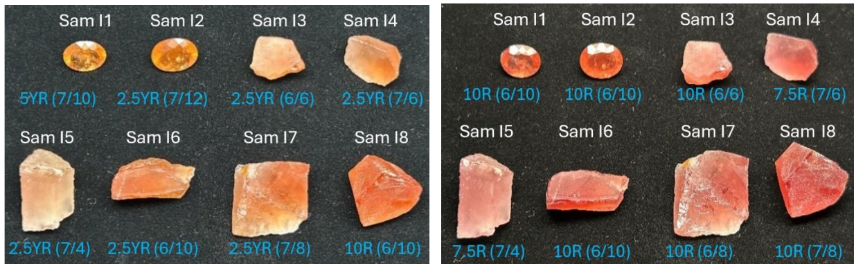
Figure 2: Comparison colors before (left) and after exposure to SWUV for 1 hour (right).
