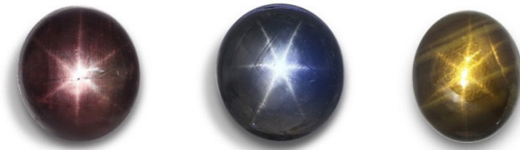
Figure 1 : Three unusual star sapphire doublets weighing 4.43 ct (pinkish-red, left), 3.56 ct (blue, middle) and 2.16 ct (yellow, right), each has a synthetic corundum dome top and a natural star sapphire base. Photo by C. Kamemakanon
