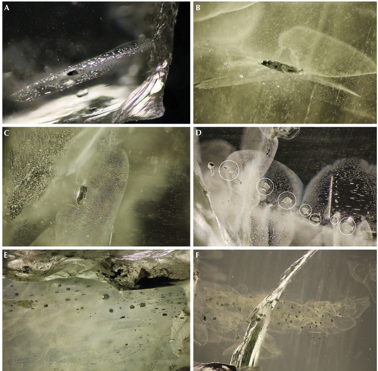
Figure 8. Internal features of Pyaung-Gaung peridot. A and B: An olivine crystal surrounded by partially healed fractures in a peridot host; field of view 3.8 mm. C–E: Olivine crystal inclusions in a peridot host; field of view 7.5 mm. F: Cluster of olivine crystals with wispy or smoky veils along with partially healed fractures; field of view 7.5 mm. Photomicrographs by M. Seneewong-Na-Ayutthaya.
