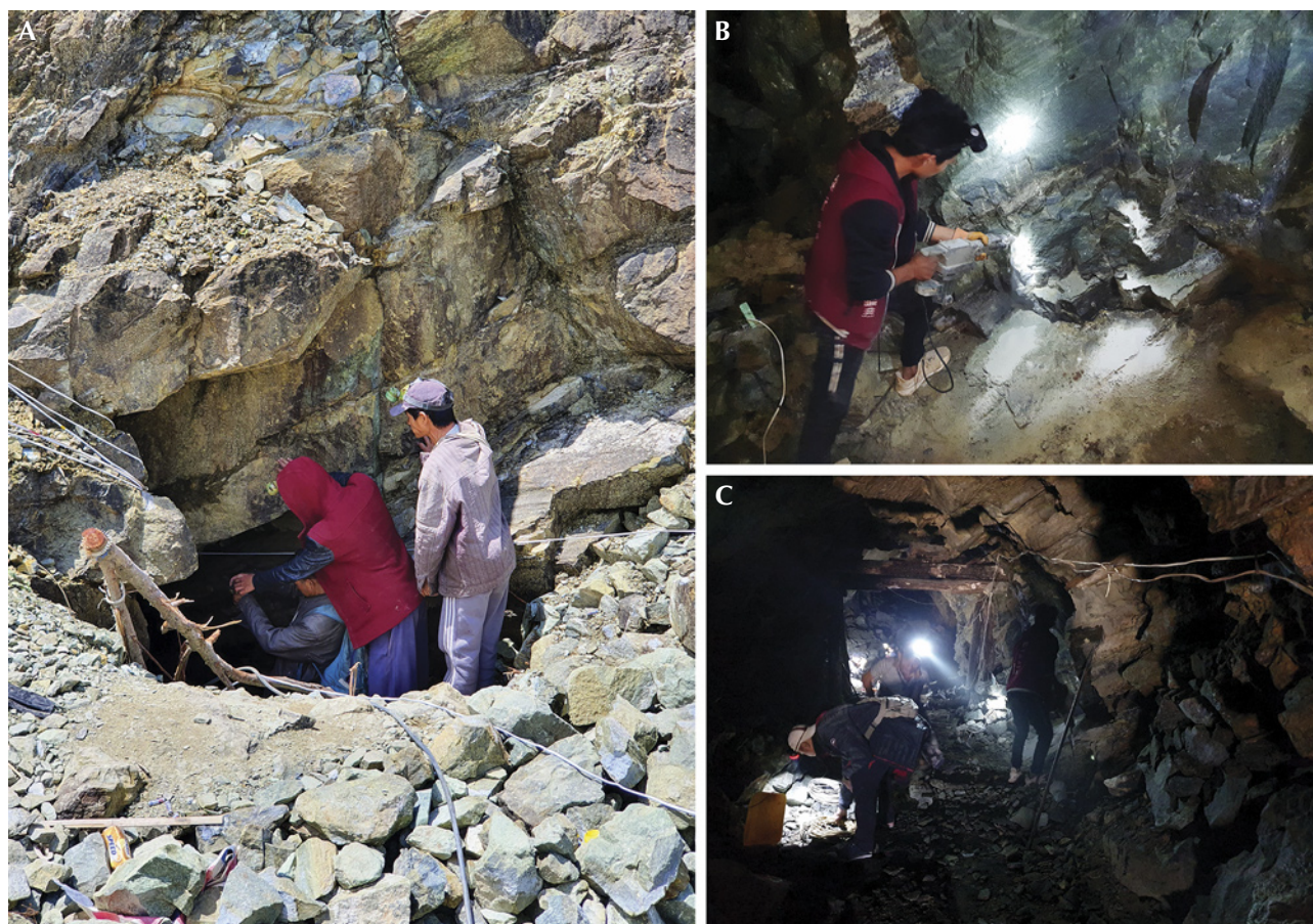
Figure 4. A: Miners entering the tunnel of an underground mine at the Pyaung-Gaung peridot deposits. B: A miner drills the rock along the tunnel wall with a pneumatic hammer to extract the peridot samples. C: Miners working in the main tunnel. Photos by M. Seneewong-Na-Ayutthaya (A) and T. Sripoonjan (B and C).
