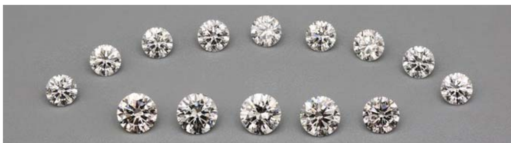
Figure 1 : These colorless samples are representative of CVD-grown diamonds from India, China, and the United State examined by GIT. They range from 0.3 to 0.1 ct. photo by M. Seneewong-Na-Ayutthaya
